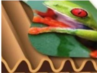
Top liner: Clay coat applied to a virgin fibre pure white Kraft board (Calliper:182 Mic/ Gloss TAPPI 75°: 35% +/- 5.00 %)
