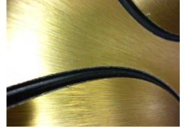
For accurate and precise manual folding of the Alupanel composite panels, resulting in a good finish, we recommend to route the rear of the panels to 2.5 mm thick, going through the exterior Aluminium layer, and some of the Polyethylene core. Normally the panel is grooved and folded 25-70 mm from the edge.
