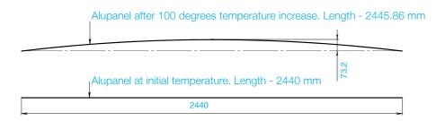
Sometimes it may happen that a substrate on which Alupanel is designed to be installed is rigidly fixed without taking thermal expansion into consideration. In this case this substrate can bow and deform causing subsequent bowing of the Alupanel which is fixed to this substrate. To prevent this, substrates on which Alupanel is going to be installed should be carefully examined.
